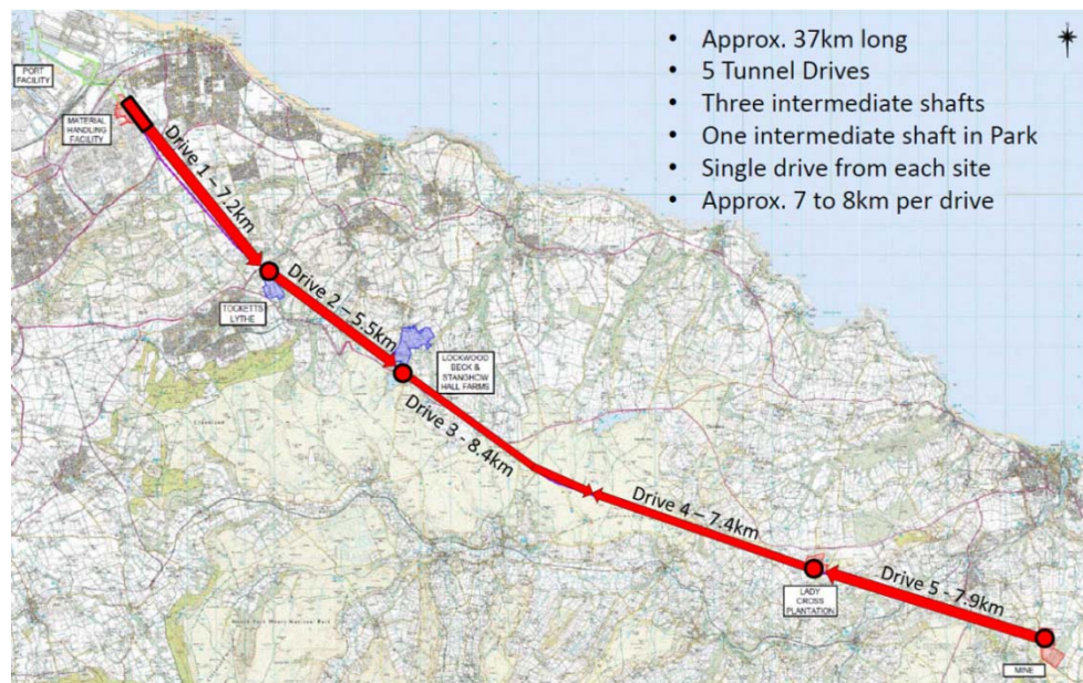
Figure 4.10 MTS Construction Strategy
